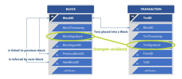
Crow's foot notation illustrating how confirmed transactions are placed into a Block. And like 'doubly-linked list', how each Block is linked to the previous and referred by the next to maintain data chronology, in order of occurrence in time.
